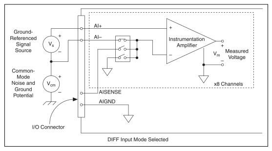
**Figure 2-5.** Differential Input Connections for Ground-Referenced Signals
